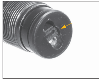
The three-shot adapter (plug) shown secured in the magazine tube.
