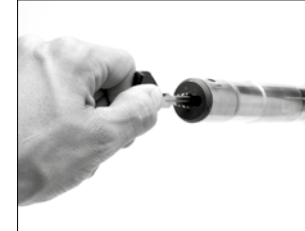
Use a key or small screwdriver to press in on the three-shot adaptor, then rotate a quarter-turn.
