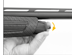
Back the assembly nut off all the way.
