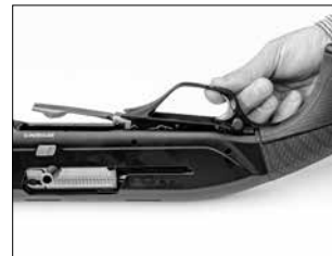
Lift the trigger group from the receiver.
