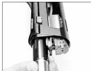
Guide the bolt slide link into its socket in the recoil spring follower.
