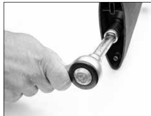
Use a socket wrench to remove the stock bolt.
